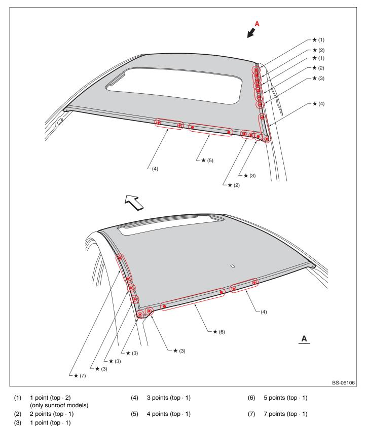
For locations marked by " $\star$ ": the welding method and the number of welding points are the same on the left and the right.
